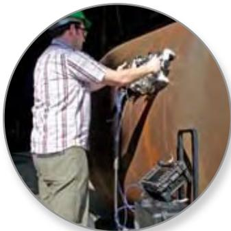
*The PV-100 and PV-200 portable systems typically feature an OmniScan, a manual scanner with water feed, and software for cost-effective inspections.*
