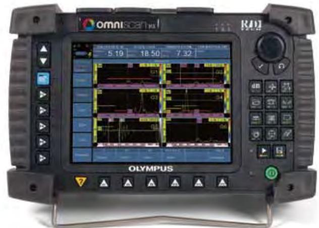
*The OmniScan MX with UT module offers TOFD (Time-of-Flight Diffraction) with conventional flaw detection and A-scan, B-scan, and C-scan displays.*
