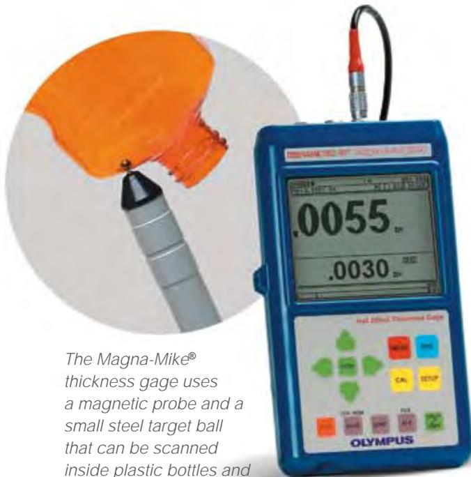
*The Magna-Mike® thickness gage uses a magnetic probe and a small steel target ball that can be scanned inside plastic bottles and non-ferrous materials.*
