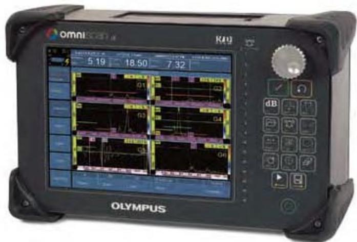
The new OmniScan iX is a high-speed industrial ultrasonic flaw detector designed for immersion or non-immersion testing of critical industrial components. This powerful, versatile instrument can be configured for 2, 4, or 8 conventional ultrasound channels.
