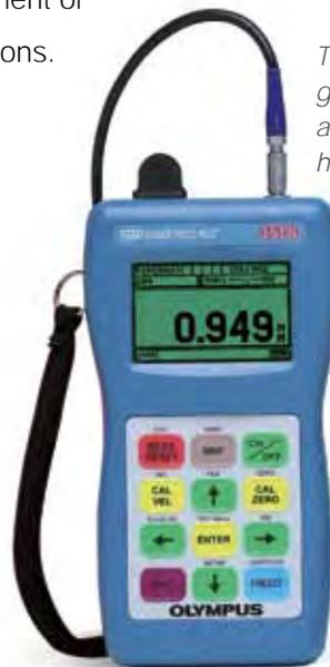
*Among the 25DL family of gages is the 25MULTI PLUS that measures three layers plus total thickness simultaneously.*
