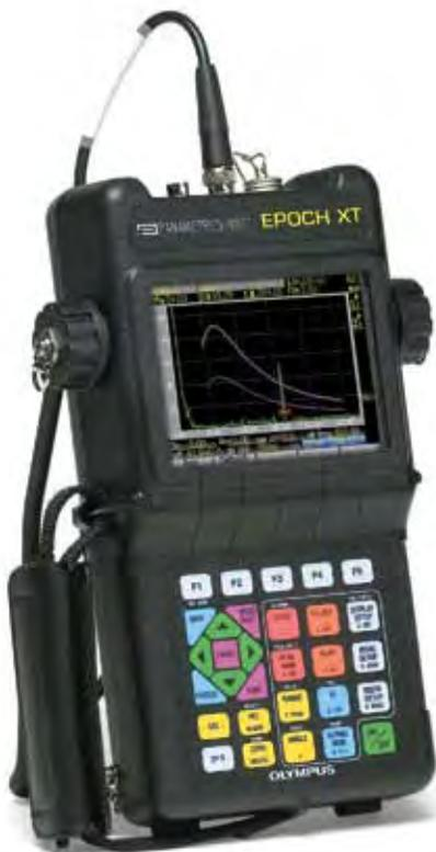
*The new EPOCH XT features a bright multi-color LCD, digital receiver filtering, versatile battery options, dual USB ports, powerful data management, and numerous software features in a compact unit with a sealed case designed to meet IP67 requirements. This unit is EN 12668-1 compliant.*
