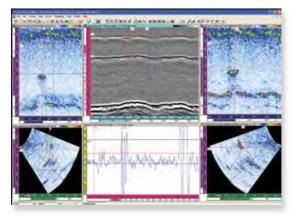
TomoView™ is a powerful and versatile software package that manages the acquisition of UT (ultrasonic testing) signals combined with the real-time imaging of these signals, as well as offline analysis of previously acquired data files. TomoView will drive the majority of R/D Tech instruments including the OmniScan units.
