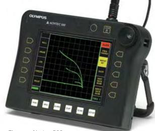
The new Nortec 500, 500S, and 500D flaw detectors offer full VGA color display, internal balance coils, VGA output, and a bidirectional USB port. The 500S also offers conductivity measurements and scanner capability. The 500D additionally offers dual frequency capability.
