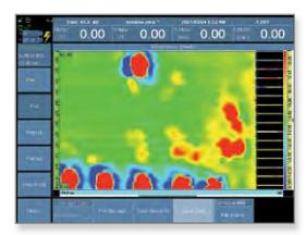
This OmniScan ECA screen shows data acquisition in a C-scan for quick and efficient defect detection.
